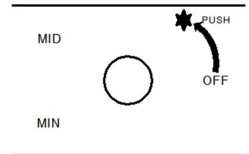
**Note: Safety valve has a stuck on each level, depress the safety valve button (D) and hold it down while adjusting the gas flow.**
