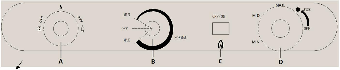
**Fig2** A: Power switch B: Thermostat knob C: Flame indicator D: Safety valve&piezoelectric igniter switch
