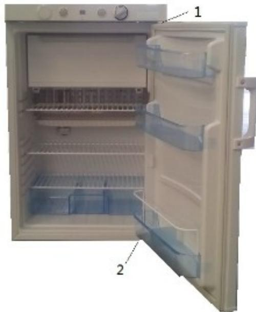
Note: As the door gasket gets pressed-in during shipment, after reversing the door the gasket might have to be reset. This will be good for seal to avoid any air escaping. If there is a gap between the cabinet and the door gasket, set the gasket by gently pulling it out to seal the gap. If necessary, you are recommended also to use the hair drier to warm the gasket to get rid of the gap.
