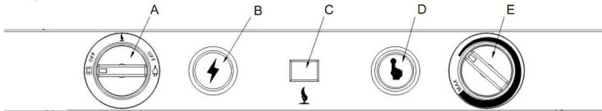
**Fig1** A: Power switch B: Pulse ignition switch C: Flame indicator D: Safety valve E: Thermostat knob
